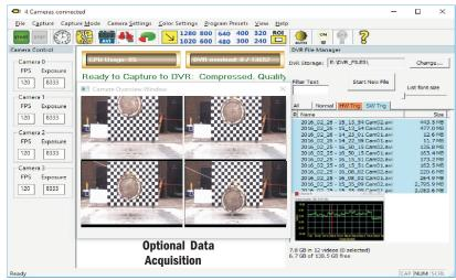
The Mega Speed MS 35K 4S camera control software is a complete software package that is included with each system. With the camera control software you can simultaneously adjust the camera settings, record the process, review the recently recorded events, edit, play back, review and transfer files without interrupting the recording process.
